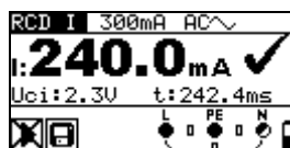
Figure 5.20: Trip-out current measurement result example
