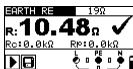
Figure 5.35: Example of earth resistance measurement result
